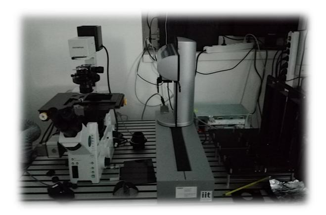
High-content system for fixed samples **Microscope:** OLYMPUS IX81-ZDC (inverted) **Objectives:** 4X/0.16 dry, 10X/0.4 dry, 20X/0.75 dry, 40X/0.60 dry **Filters for:** DAPI, EGFP, RFP, CY5, T-Red **Transmission mode:** Bright-field **Camera:** Hamamatsu ORCA-ER B/W CCD **Software:** Scan^R Acquisition (version 2.4.0.13)
